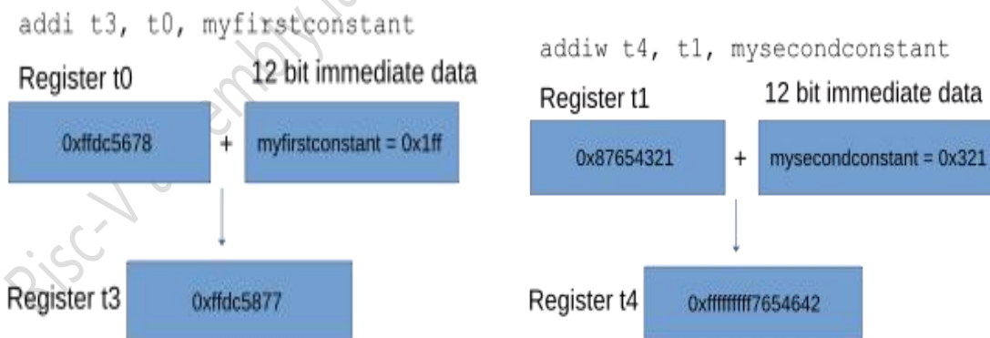
Figure 4-4 Illustrating the ADD and ADDIW instructions
